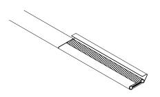
**B** Remove overjacket from the heater cable.
