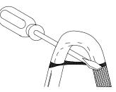
• While bending the heater cable, work it through the braid opening.
