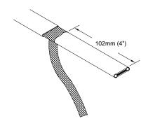
**6** At the bulge, separate the braid to make an opening.
