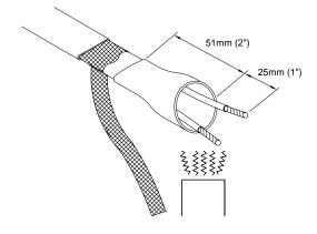
Slide one 12mm (0.5") diameter, 51mm (2") length shrink tube over both pigtail leads leaving approximately 25mm (1") of each pigtail lead exposed. Shrink with heat gun until completely shrunk.
